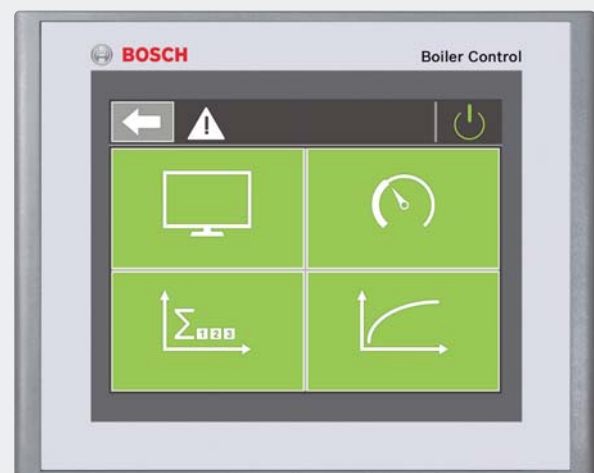
2 nd level: Selection menu with four areas: operation monitor, function values, consumption values and measurement values
