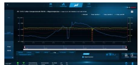
From all the variables recorded, configurable statistics display with freely selectable timescale and storage of your own display configurations.
