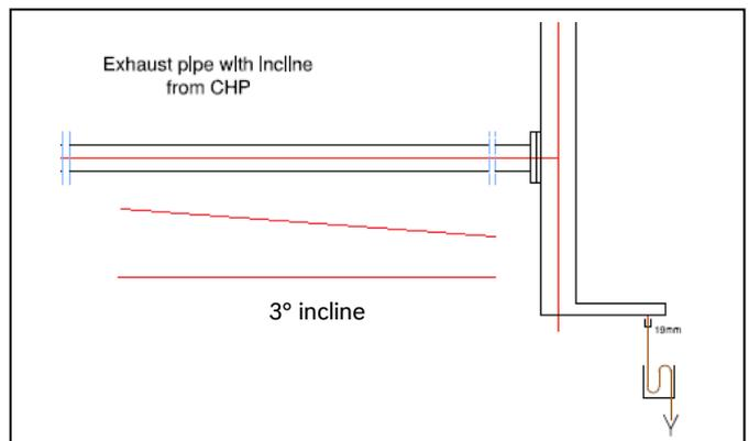
Fig.3: 3° incline towards the primary condensate drain point
