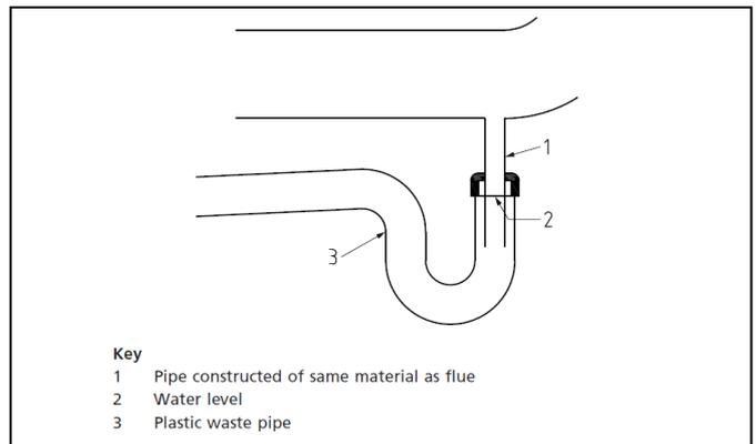
Fig.2: Detail of trap arrangement showing the trap connected immediately below the spigot from the flue system drain.
