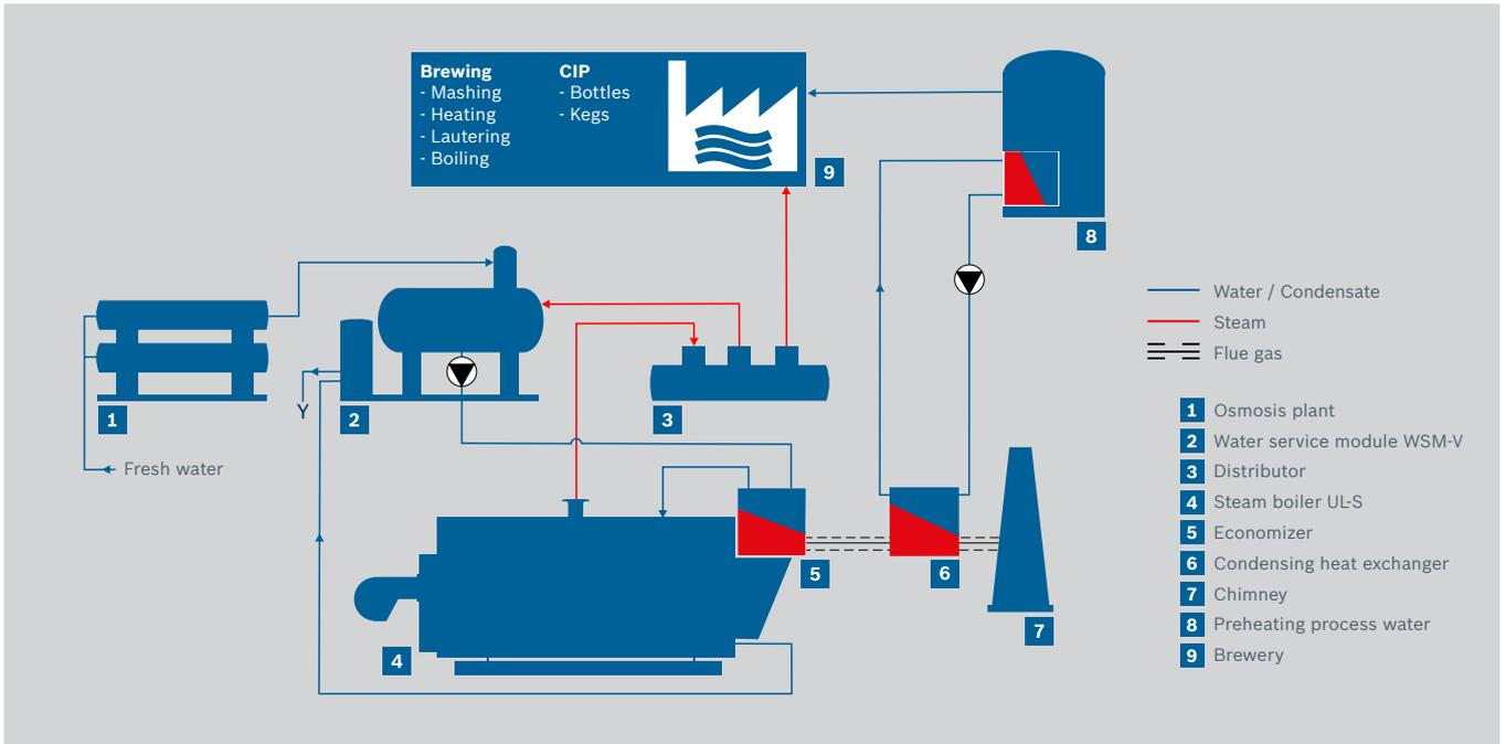
Simplified schematic diagram of the steam boiler plant at the Pivovar Klášter brewery.
