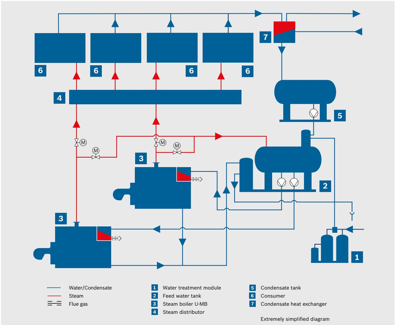
System diagram steam boiler with appropriate plant technology for heat recovery, water treatment and condensate return.
