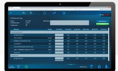
Digital boiler log books offer progress in this regard. Tendencies or critical deviations are often detected too late or not at all during stipulated water-chemical measurements and system checks. A digital boiler log book analyses the measured values entered and assists the user with individual information and suggested solutions.
