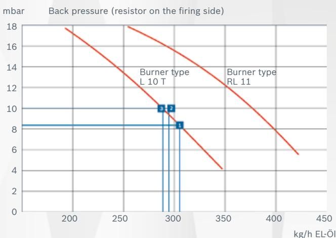
Graphic: Burner grid with maximum output graphs
