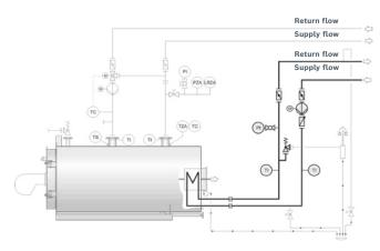
Figure 5: Hydraulic circuit for optimal use of condensing technology.
