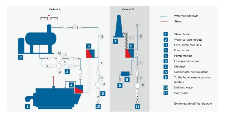
Figure 7: Simplified diagram of a high-pressure boiler system with two flue gas heat exchanger stages (economiser/flue gas condenser).
