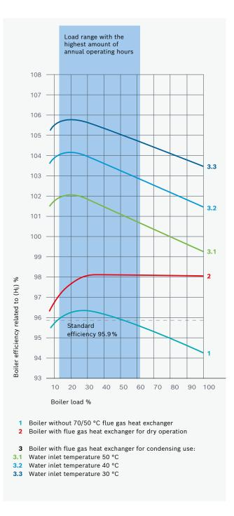
Figure 2: Efficiency curves for condensing technology (using a hot water boiler with gas combustion as an example).
