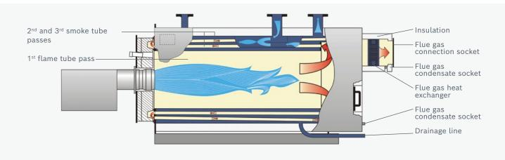
Figure 3: Cross-section of a Bosch heating boiler (UT-L) with an integrated flue gas heat exchanger.
