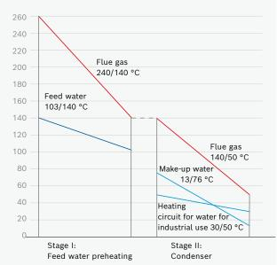
Figure 6: Two-stage flue gas heat recovery with flue gas/ water temperature at 100 % load.
