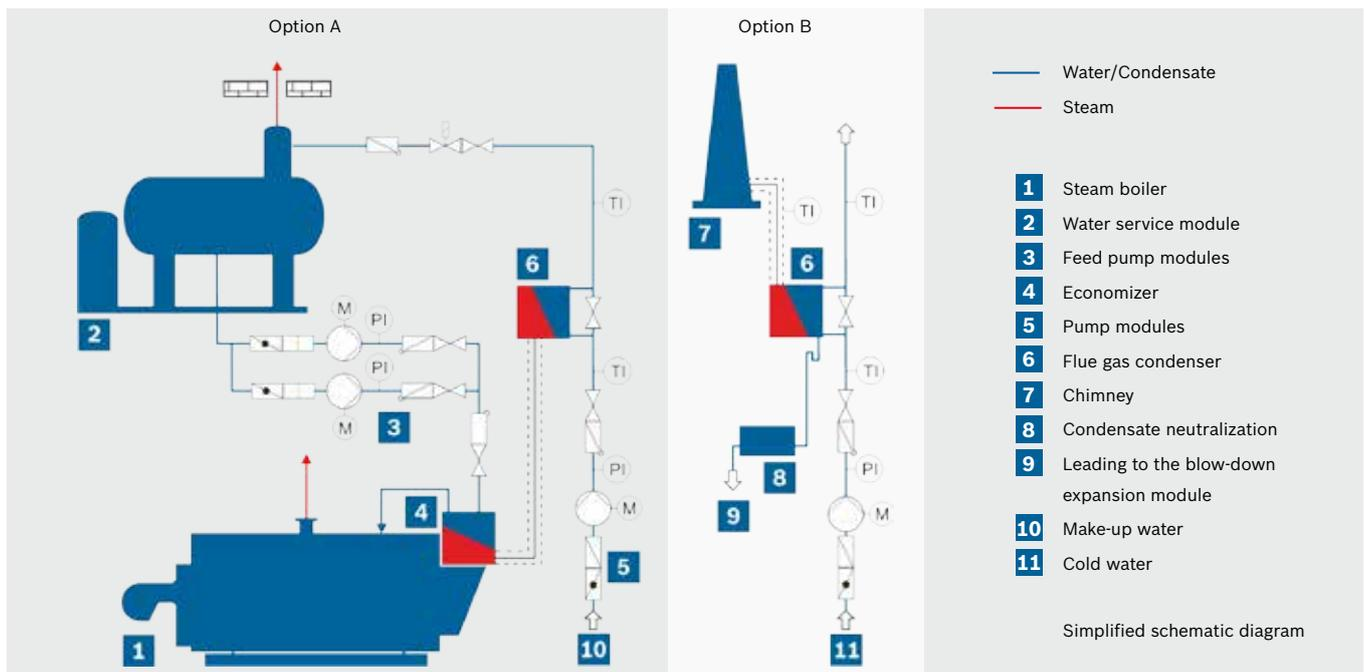
Figure 2: Steam generator with two-stage operation – economizer/flue gas condenser; capacity optimization of up to 15 % of the boiler capacity
