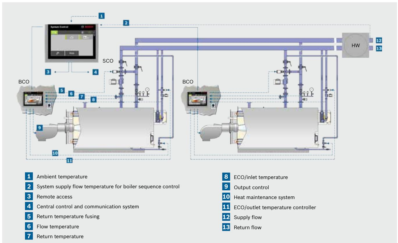
Figure 4: Hot water boiler system with hydraulic separator controlled on the basis of atmospheric conditions
