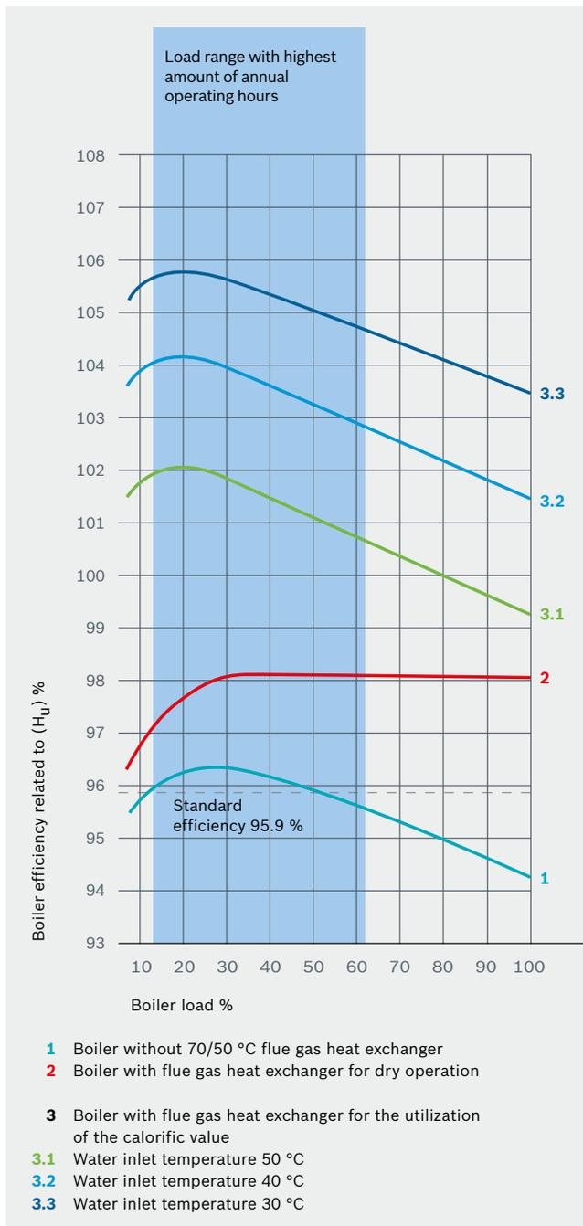
Graphic 2: Efficiency graphs for UNIMAT hot water boilers with 70/50 °C boiler supply/return flows
