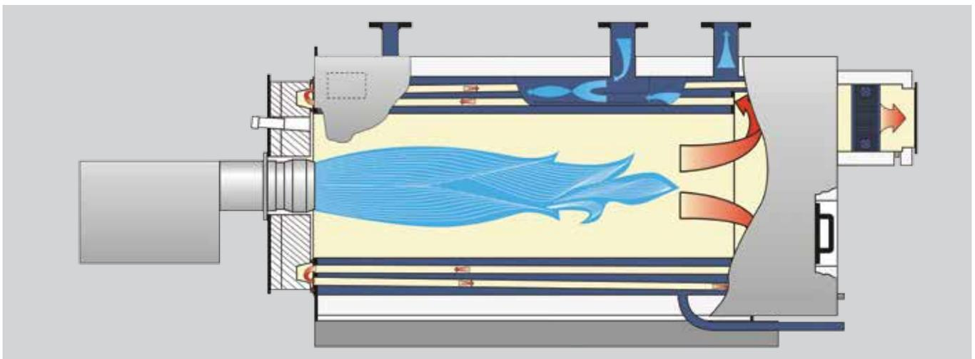
Figure 3: Single-flame smoke-tube hot water boiler designed according to the three-pass principle with flue gas heat exchanger
