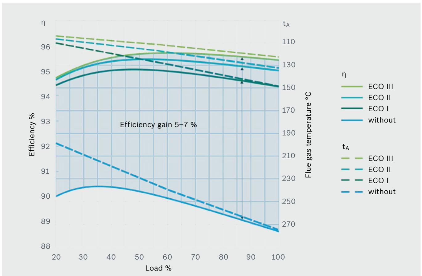
Graphic 1: Achievable capacity optimisation from flue gas heat exchangers for „dry“ operation
