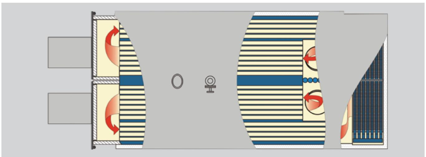
Figure 1: Three-pass double-flame smoke-tube boiler with separate flue gas ducts for independent burner operation and integrated economizer for heating feed water
