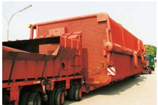
Figure 2: 100 MW hot water – water tube boiler during transport
