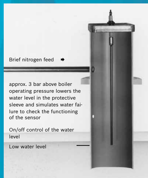
Figure 2: simple electrode – mandatory daily test through blowing in nitrogen.
