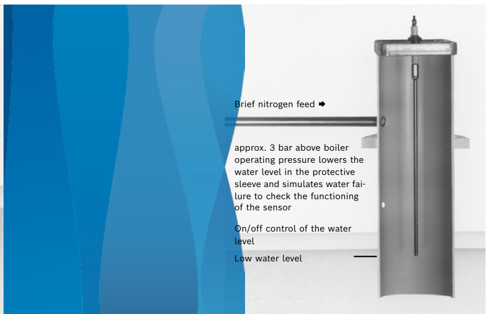
Figure 2: simple electrode – mandatory daily test through blowing in nitrogen.
