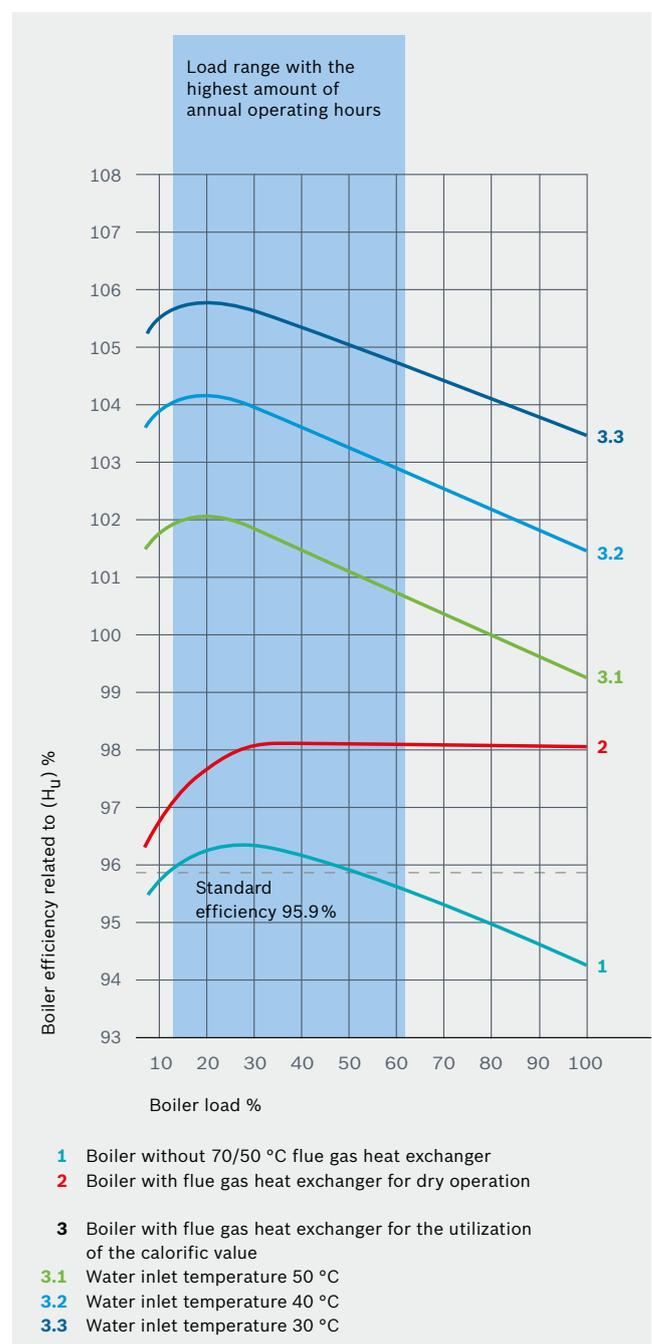
Graphic 2: Efficiency curves for the utilization of the calorific value (example hot water boiler with gas firing system)
