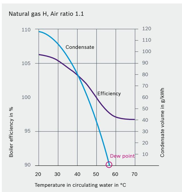
Graphic 1: Influence of the temperature of circulating water on boiler efficiency and condensate volume for natural gas (Ruhrgas)
