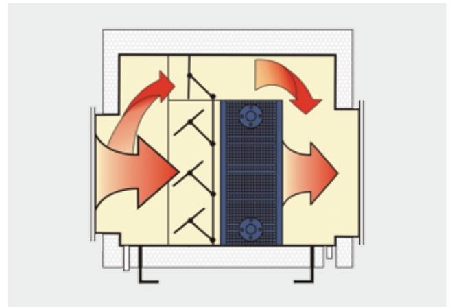
Figure 2: Flue gas heat exchanger for separate installation and retrofitting
