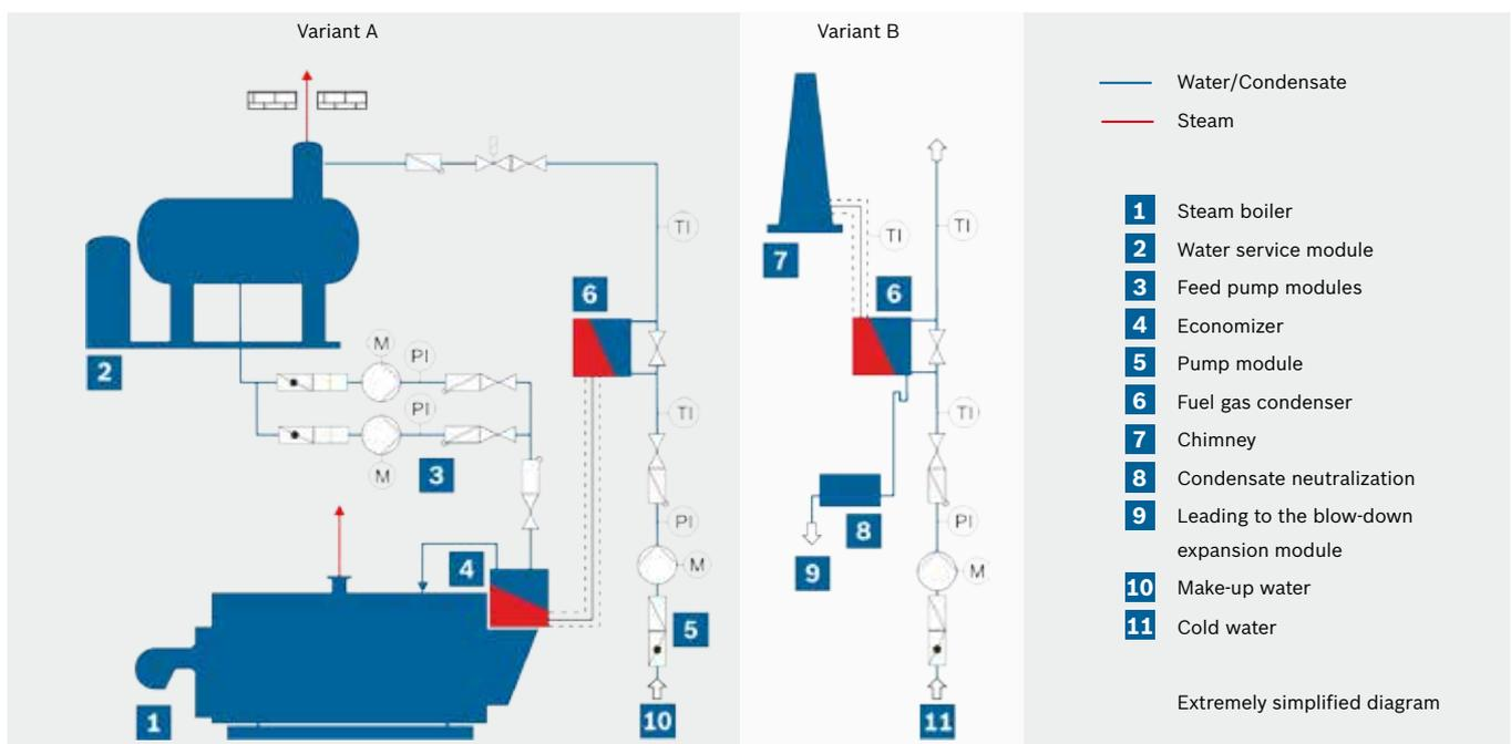
Figure 4: Block diagram of a high-pressure steam boiler system with two flue gas heat exchanger stages (economizer/flue gas condenser)
