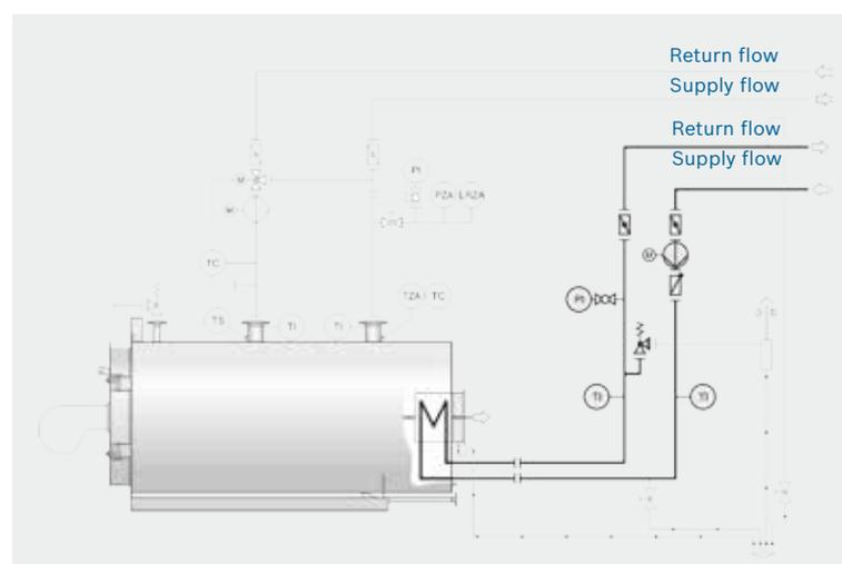
Figure 3: Hydraulic circuit for optimum utilization of the calorific value
