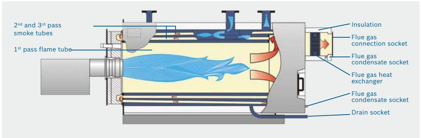
Figure 1: Sectional drawing of the UNIMAT heating boiler with integrated flue gas heat exchanger
