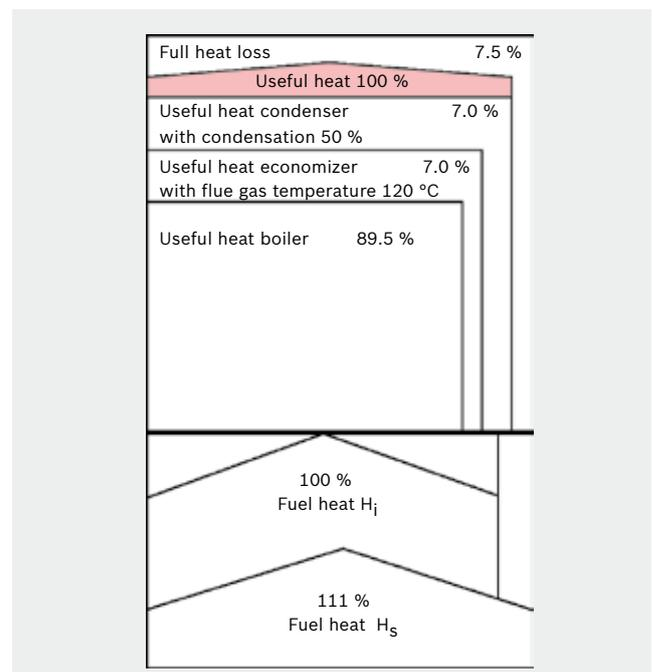
Graphic 4: Thermal balance of a steam generator with calorific value technology
