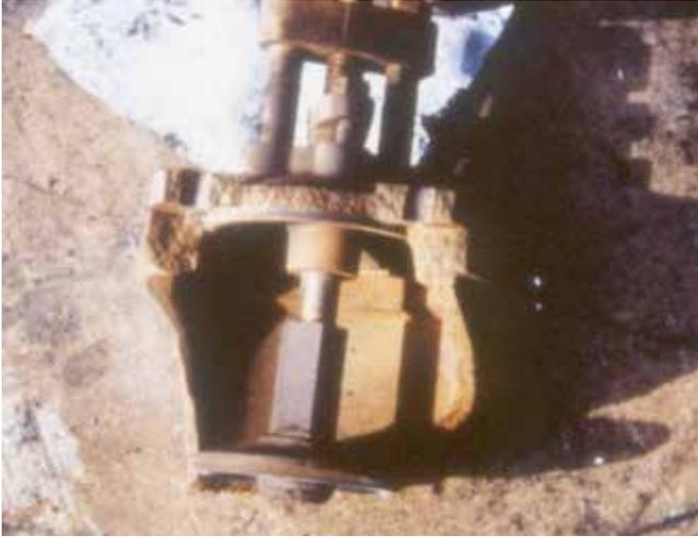
Figure 2: Valve destroyed by water impact
