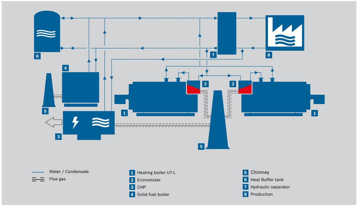
Simplified piping diagram of the plant.
