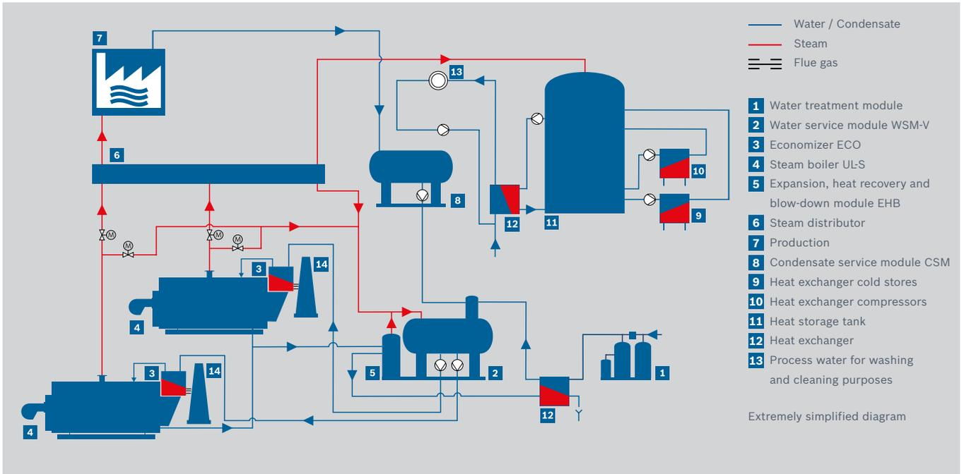
System diagram steam boiler with appropriate plant technology for heat recovery, water treatment and waste heat utilisation involving the compressors and cold stores.
