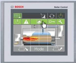
**1<sup>st</sup> level:** Start page with the new button “Condition Monitoring”
