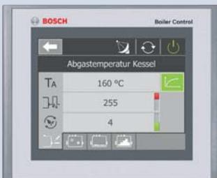
**3<sup>rd</sup> level:** Detailed view with new optical display in form of “traffic light function”
