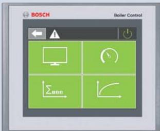
**2<sup>nd</sup> level:** Selection menu with four areas: operation monitor, function values, consumption values and measurement values
