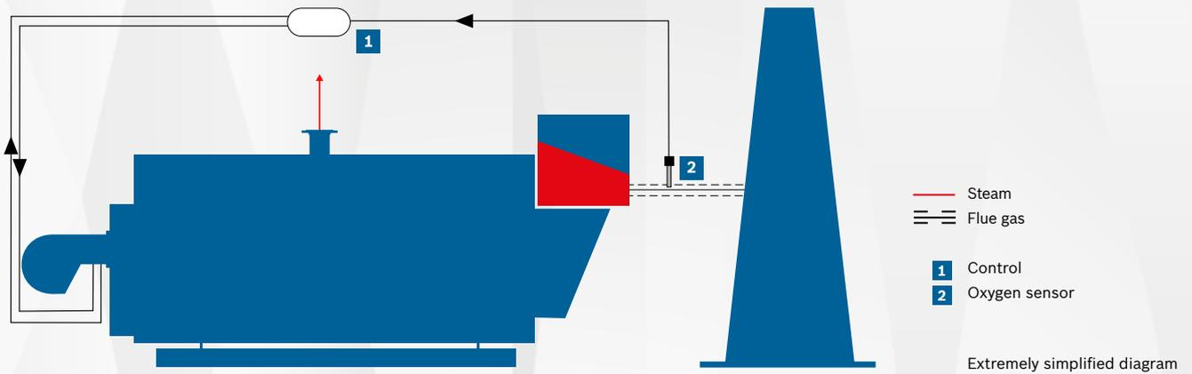
Schematic diagram oxygen control.
