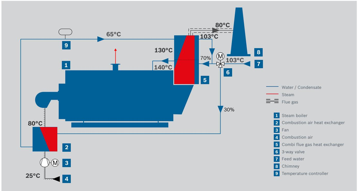
Simplified hydraulic diagram of the Bosch air preheating system at Rauch Fruchtsäfte.
