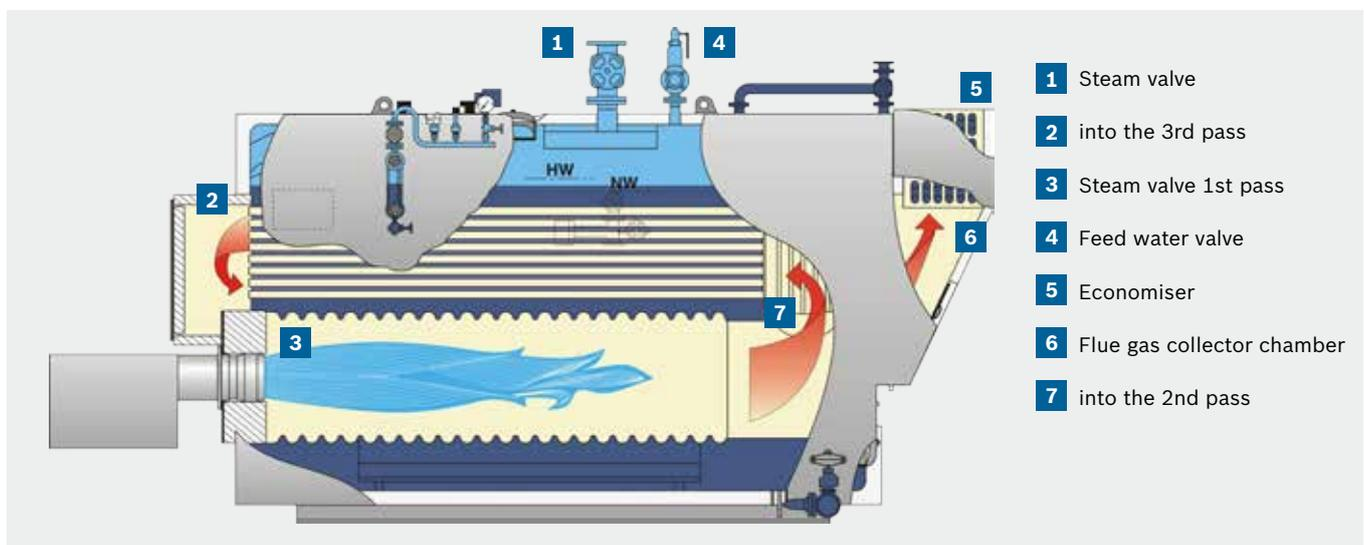
Section through a steam double-flue boiler in three-pass compact technology and piggy-back-welded Economiser. The two flue gas channels are separate right through to the flue gas connection. This means that the burners can be operated individually.
