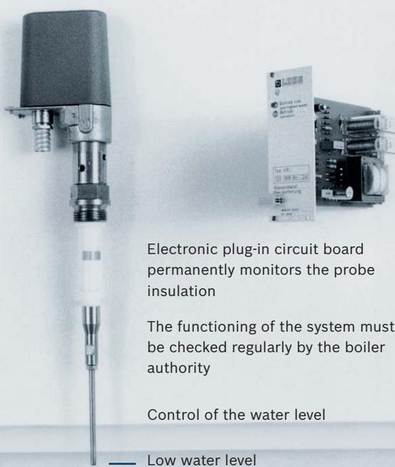
Figure 4: Self monitoring probe water level monitor – no maintenance, no functional test required
