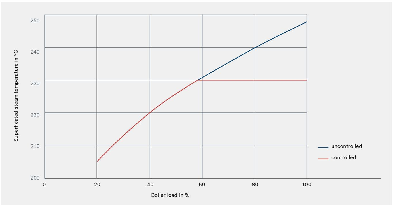
Graphic 2: Superheated steam diagram for controlled and uncontrolled operation
