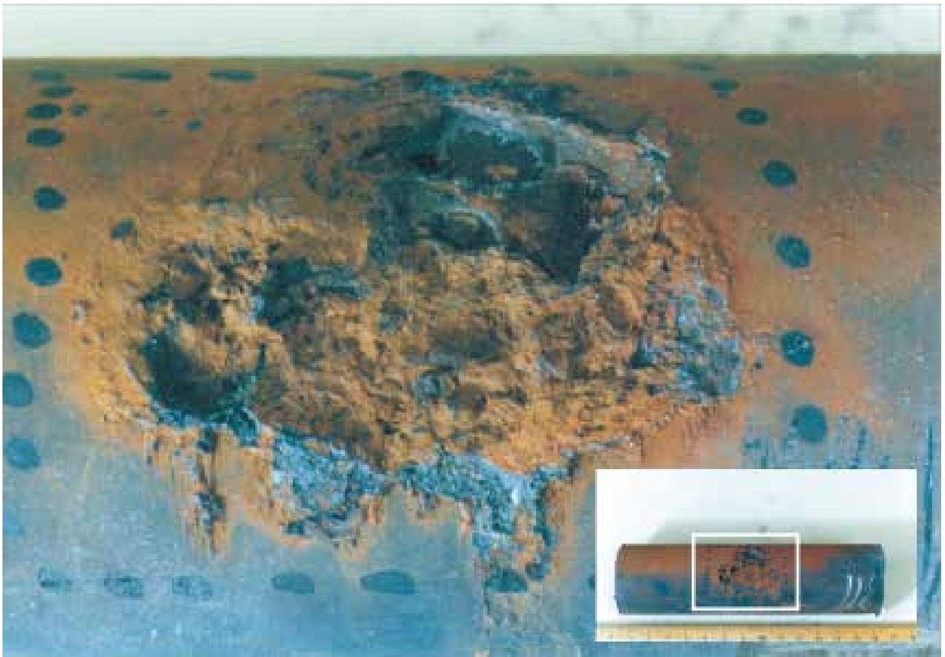
Figure 3: Oxygen attack on a cut-out smoke tube
